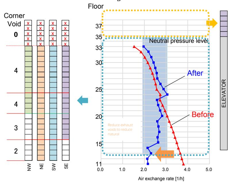
Fig. 22 CONCEPT DESIGN STAGE SIMULATION (FLOW NETWORK CALCULATION)
