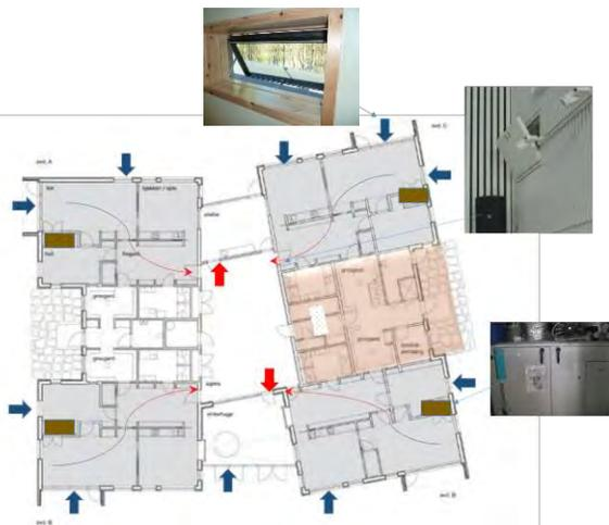
Fig. 5 NATURAL AND MECHANICAL VENTILATION AT SOLSTAD. MOTOR CONTROLLED WINDOW, HATCHES BETWEEN WING AND AGORA AND MECHANICAL VENTILATION
