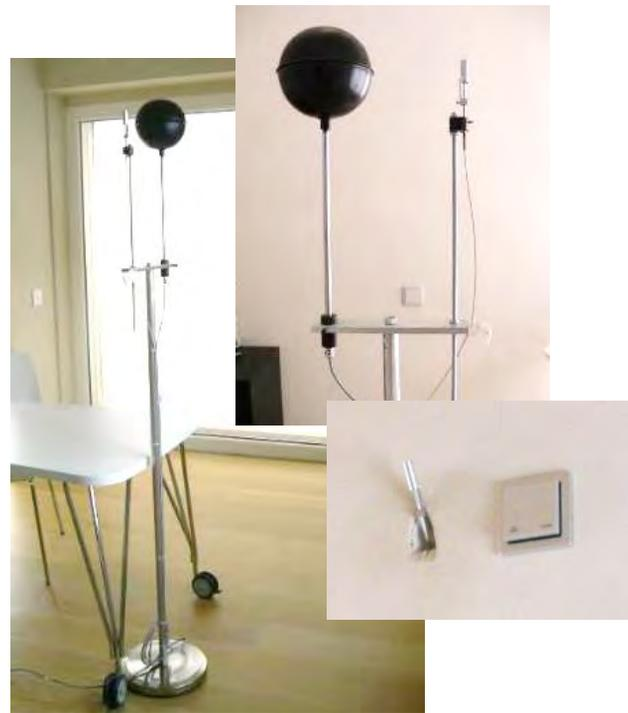
**Fig.21** EXAMPLE OF INDOOR SENSORS INSTALLED TO MEASURE OPERATIVE AND AIR TEMPERATURE, RH, CO2 CONCENTRATION
