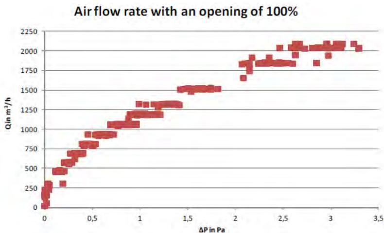
**Fig. 18** MEASURED AIR FLOW RATES THROUGH FREE AREA OF ROOF WINDOW
