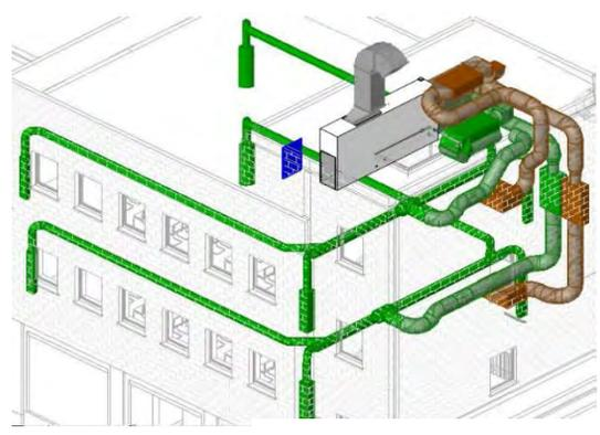
Fig. 6 VISUALISATION OF AIR DISTRIBUTION (SUPPLY IN GREEN, RETURN IN BROWN)
