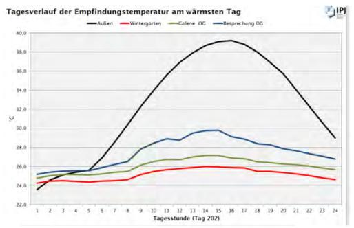
**Fig. 14** ZONE TEMPERATURE ON THE HOTTEST DAY, TAS 9.2, DESIGN STAGE SIMULATION, SOURCE: IPJ INGENIEURBÜRO P. JUNG GMBH.
