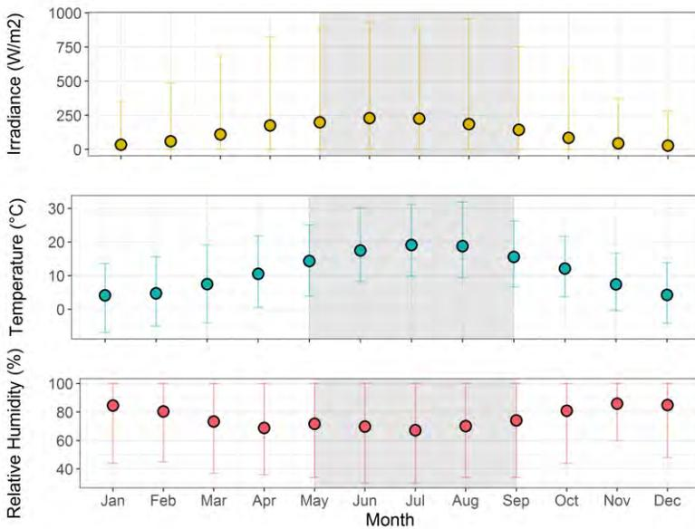
Fig.2 MEAN EXTERNAL CONDITIONS IN TRAPPES, FRANCE USING A TMY3 (SHADED AREA IN GREY INDICATES COOLING SEASON)
