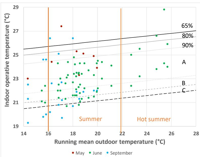
**Fig. 25** EVALUATION ADAPTIVE TEMPERATURE LIMITS METHOD
