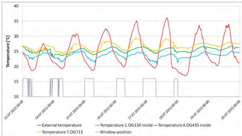
Fig. 18 INTERNAL TEMPERATURE PROFILE ROOMS 130, 435, 713 IN JULY 2015
