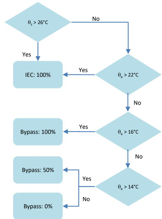
**Fig. 12** CONTROL STRATEGY FLOWCHART AHU DURING OCCUPANCY
