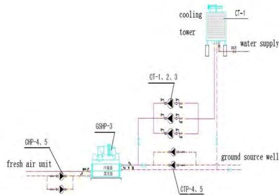
Fig. 6 PROCESS DIAGRAM OF FRESH AIR SYSTEM
