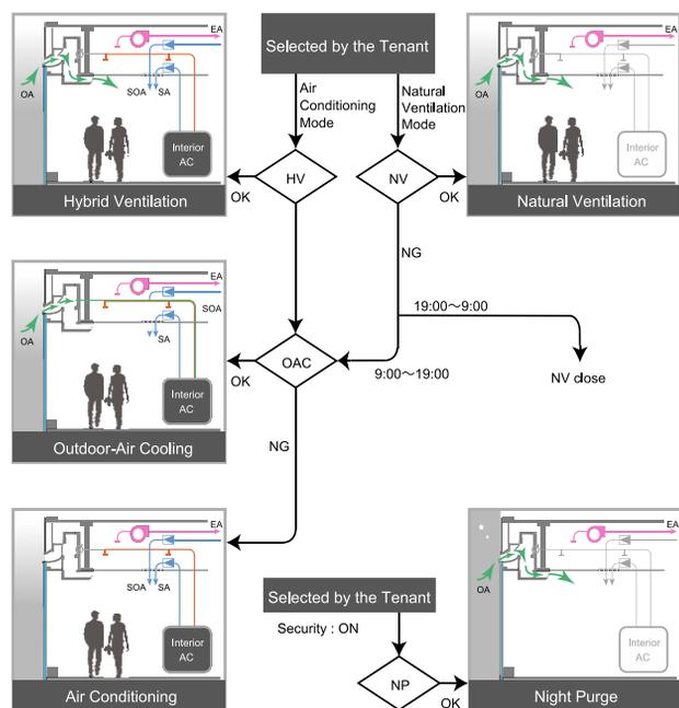
Fig. 18 AUTOMATED VENTILATOR AND AHU CONTROL FLOWCHART
