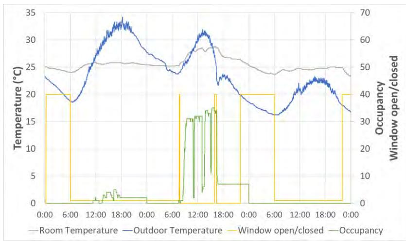
**Fig. 21** INDOOR TEMPERATURE AND OPERATION WINDOWS DURING AN EXTREMELY WARM PERIOD 21-23 JUNE 2017
