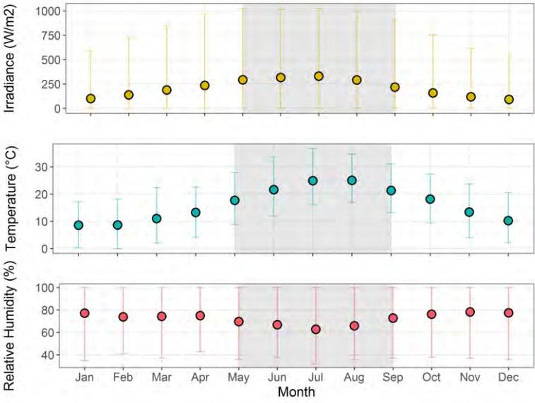
**Fig.2** MEAN, MAXIMUM AND MINIMUM EXTERNAL CONDITIONS IN MASCALUCIA USING TMY3 FROM METEONORM 7 (COOLING SEASON SHOWN SHADED)
