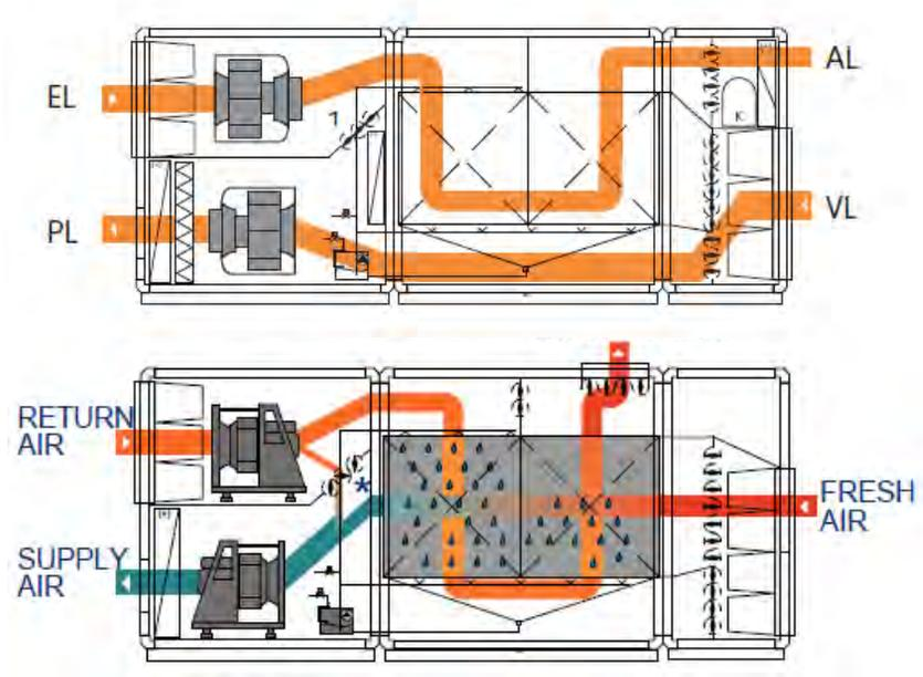
Fig. 10 SCHEME OF MODULAR BYPASS AND INDIRECT EVAPORATIVE COOLING
