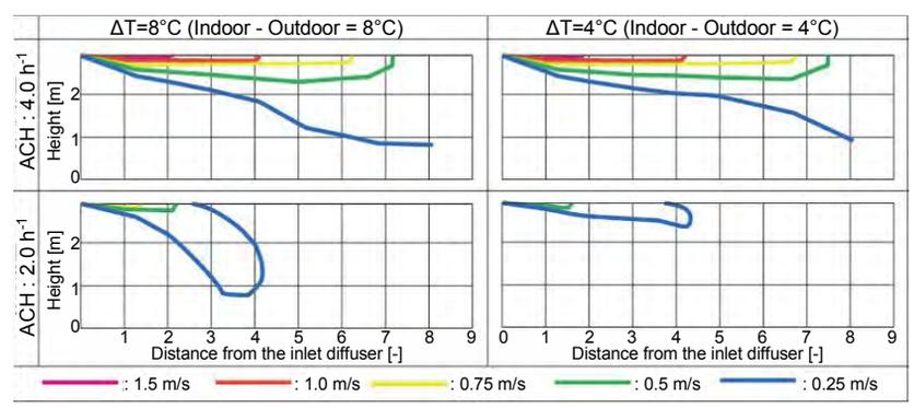
Fig.15 VELOCITY CONTOUR LINES AROUND NV INLET DIFFUSER
