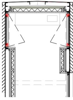
Fig. 8 CHIMNEY WITH OUTLET TOP HUNG WINDOWS
