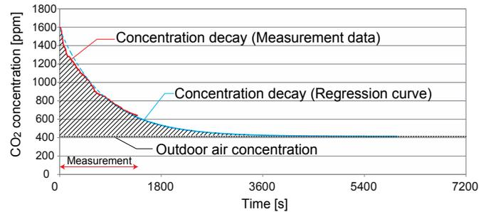
Fig. 27 CALCULATION OF LOCAL MEAN AGE OF AIR BASED ON MEASURED CO<sub>2</sub> CONCENTRATION
