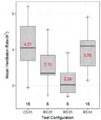
**Fig. 20** ACR MEASURED IN RETROFIT AND EXISTING BUILDING DURING SUMMER 2013
