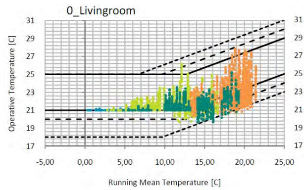
**Fig. 15** OVERHEATING EVALUATION BASED ON EN 15251
