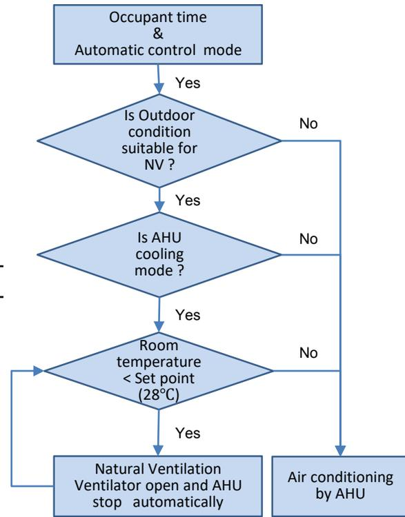
**Fig. 18** AUTOMATED VENTILATOR AND AHU CONTROL FLOWCHART
