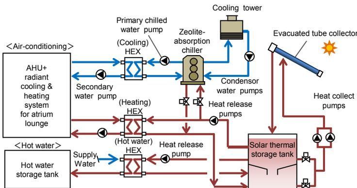
Fig. 8 MULTI-USE SOLAR HEATING AND COOLING SYSTEMS
