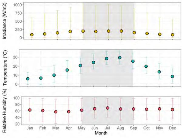
Fig.3 MEAN, MAXIMUM AND MINIMUM EXTERNAL CONDITIONS IN CORK AIRPORT USING TMY3 (COOLING SEASON SHOWN SHADED)
