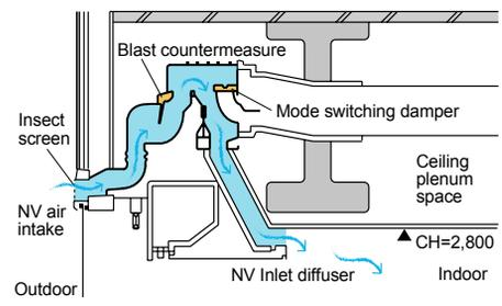
Fig.13 SCHEMATIC OF THE NV INLET DIFFUSER
