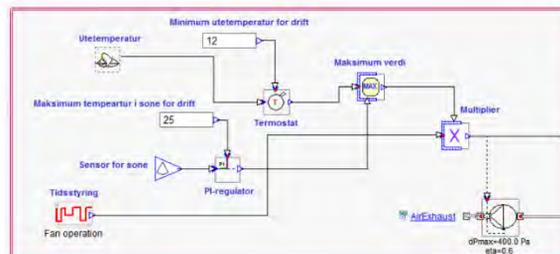
Fig. 10 EXHAUST VENTILATION CONTROL
