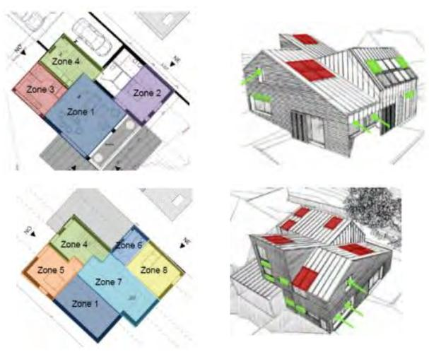
Fig. 9 NATURAL VENTILATION SYSTEM: ZONES, INLET AND OUTLET WINDOWS
