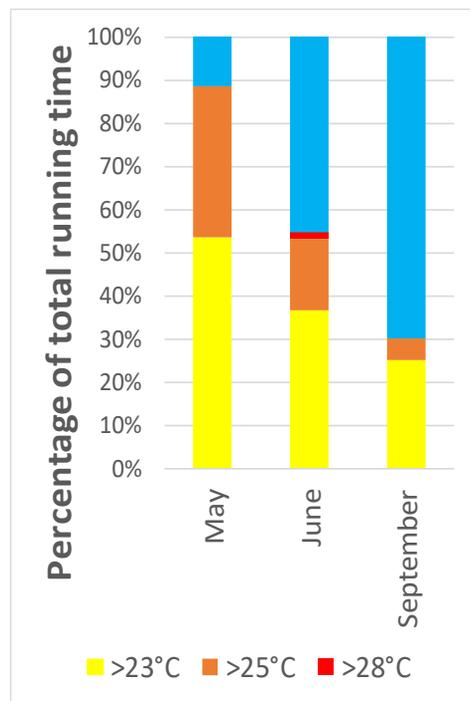
**Fig. 24** PERCENTAGE OF HOURS ABOVE THRESHOLD VALUES FOR INTERNAL TEMPERATURES IN LECTURE ROOM ON 1<sup>ST</sup> FLOOR MAY-SEPTEMBER 2017
