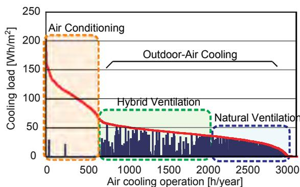
Fig. 19 COOLING LOAD DURATION CURVE
