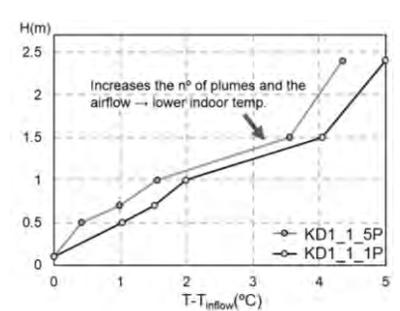
**Fig. 16** SHORT-TERM MEASUREMENTS : NUMBER OF PLUMES IMPACT ON INDOOR AIR TEMPERATURE.
