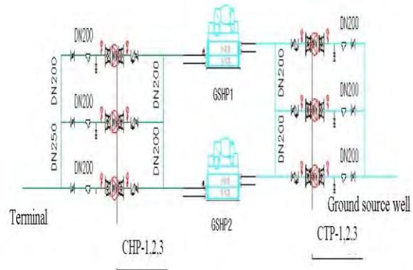
Fig. 5 PROCESS DIAGRAM OF RADIATION SYSTEM
