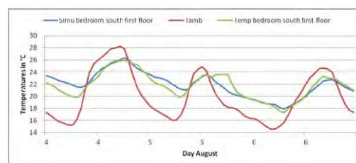
Fig. 19 COMPARISON BETWEEN SIMULATED AND MEASURED INDOOR TEMPERATURES
