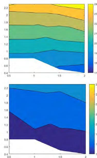
Fig. 20 air temperature profile in the room at the start (above) and after 60 min for cross ventilation
