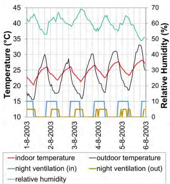
Fig. 22 MEASURED INDOOR AND OUTDOOR TEMPERATURE, INDOOR RELATIVE HUMIDITY AND OPERATION OF VENTILATION OPENINGS DURING A HEAT WAVE IN 2003
