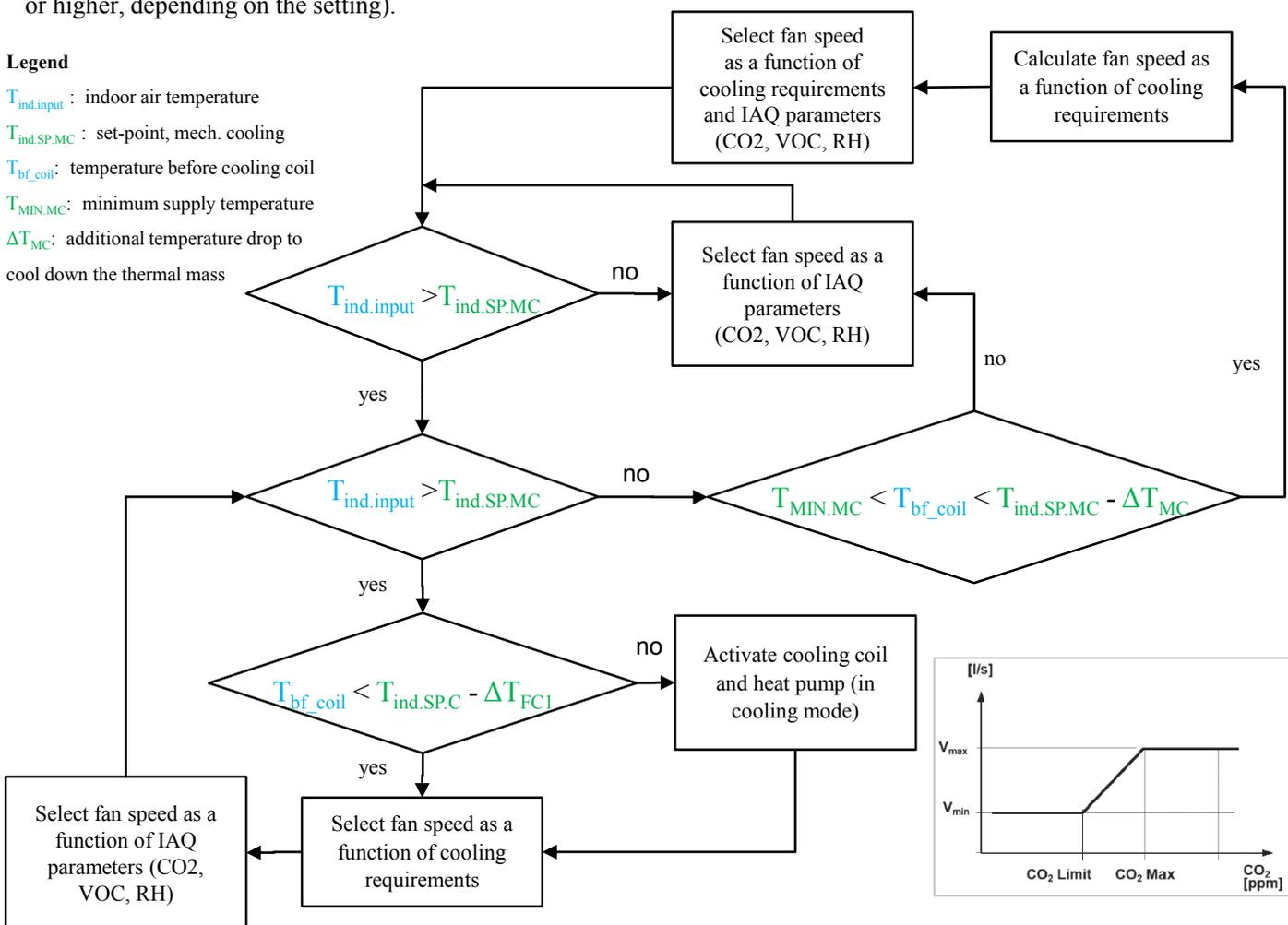
**Fig. 11** CONTROL STRATEGY. BOTTOM RIGHT: VARIATION OF THE VOLUMETRIC FLOW RATE AS A FUNCTION OF CO<sub>2</sub> CONCENTRATION LEVEL
