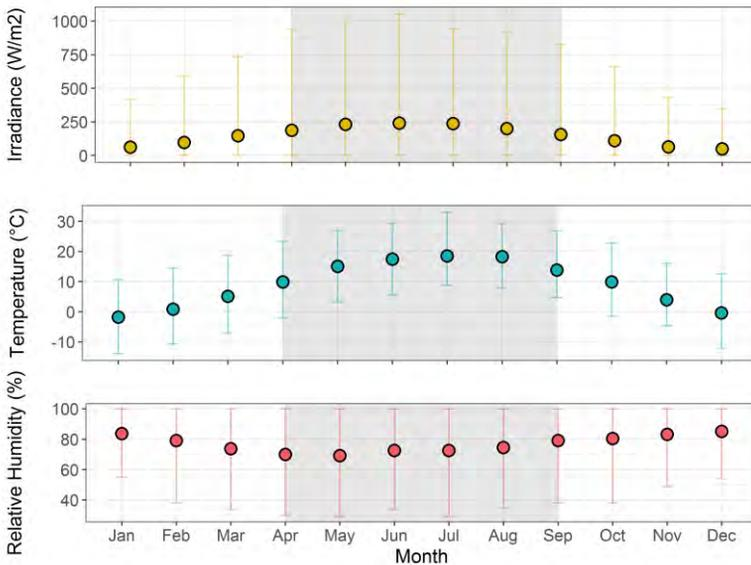
**Fig.2** MEAN, MAXIMUM AND MINIMUM EXTERNAL CONDITIONS AT INNSBRUCK UNIVERSITY USING TMY3 FROM METEONORM 7 (COOLING SEASON SHOWN SHADED)
