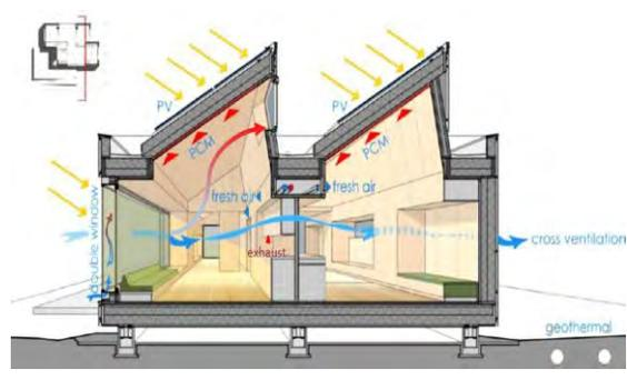
Fig.9 VENTILATIVE COOLING PRINCIPLE
