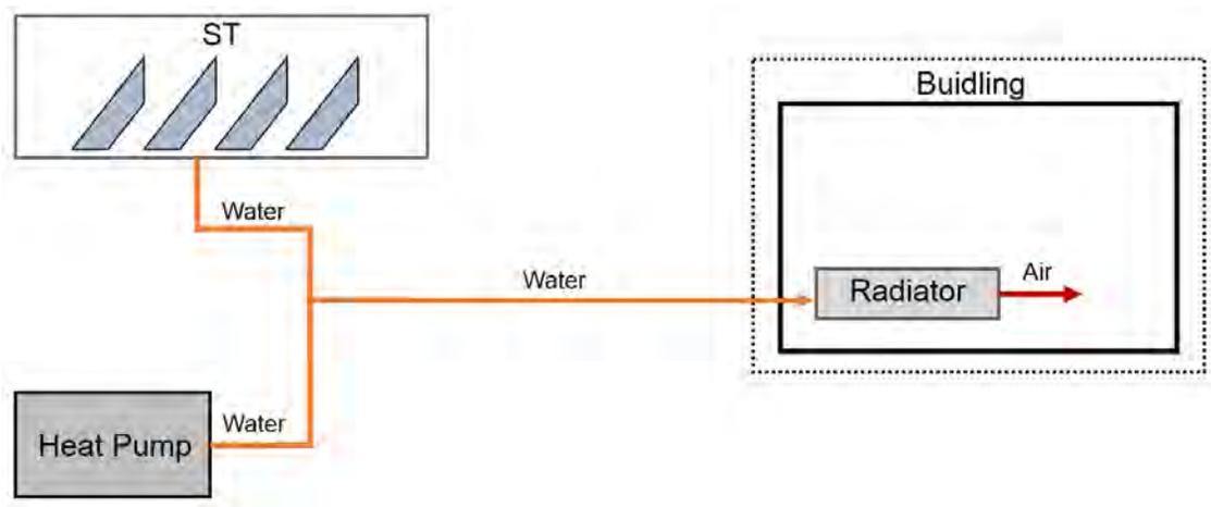
Fig.6 SCHEMATIC DESCRIPTION OF CML KINDERGARTEN HEATING SYSTEM
