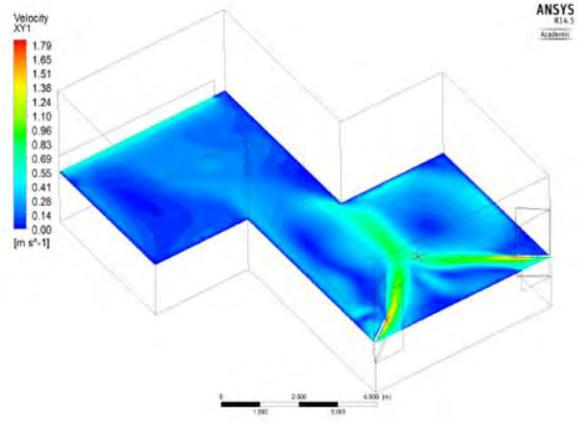
Fig. 17 EXAMPLE HORIZONTAL AIR VELOCITY VARIATION AT HEIGHT 1.5M. INLET VELOCITY 0.5M/S
