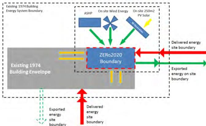
Fig.8 SCHEMATIC DESCRIPTION OF ZERO2020 TESTBED INFRASTRUCTURE
