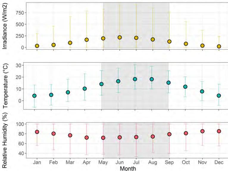
**Fig.2** MEAN, MAXIMUM AND MINIMUM EXTERNAL CONDITIONS IN WAREGEM USING TMY3 FROM METEONORM 7 (COOLING SEASON SHOWN SHADED)
