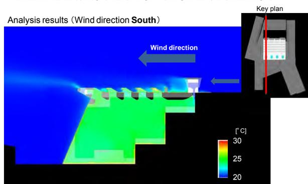
**Fig. 22** DETAIL DESIGN STAGE SIMULATION: INDOOR THERMAL ENVIRONMENT FOR NATURAL VENTILATION
