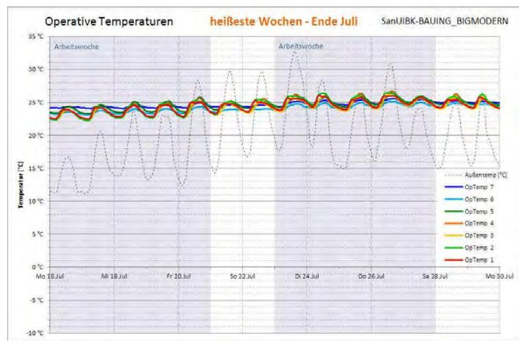
**Fig. 14** ZONE TEMPERATURES DURING HOTTEST WEEKS IN JULY, RESULTS FROM DESIGN STAGE SIMULATION, SOURCE: PASSIVHAUS INSTITUT
