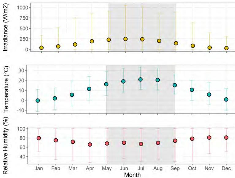
**Fig.2** MEAN, MAXIMUM AND MINIMUM EXTERNAL CONDITIONS AT ERNSTBRUNN USING TMY3 FROM METEONORM 7 (COOLING SEASON SHOWN SHADED)
