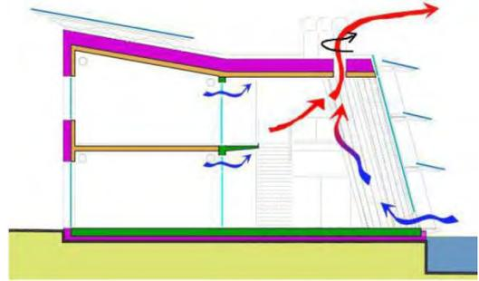
Fig. 8 VENTILATIVE COOLING PRINCIPLE, SOURCE: ARCHITEKTURBÜRO REINBERG ZTGMBH
