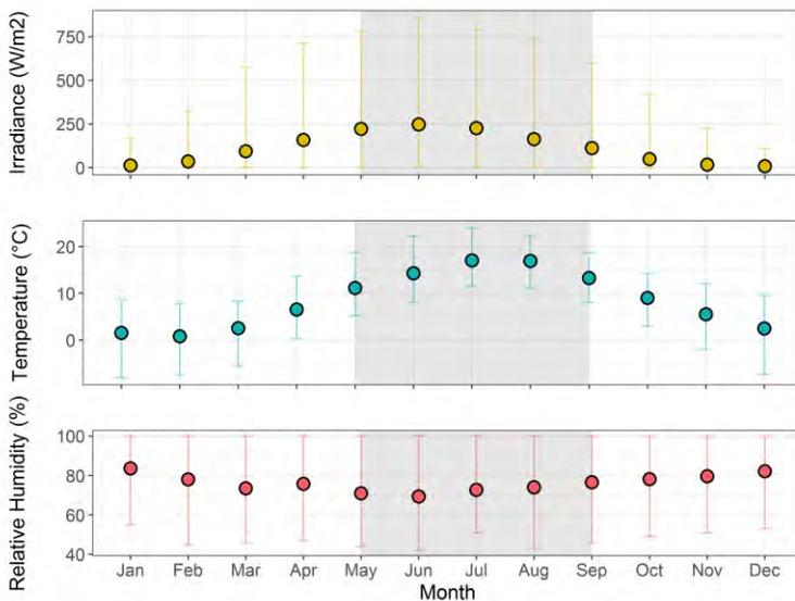
**Fig.2** MEAN, MAXIMUM AND MINIMUM EXTERNAL CONDITIONS IN LARVIK AIRPORT USING TMY3 FROM METEONORM 7 (COOLING SEASON SHOWN SHADED)
