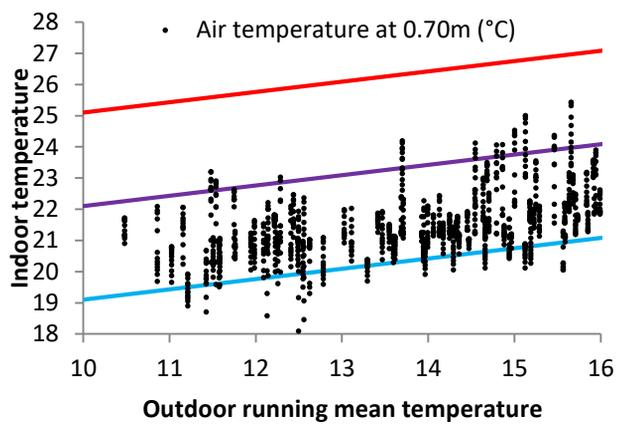
Fig. 10 – MEASURED AIR TEMPERATURE AND RH IN COMPARISON TO THERMAL COMFORT LIMITS
