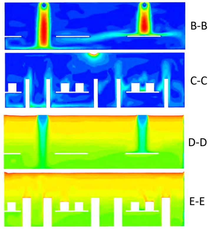
**Fig. 17** AIR VELOCITY AND AIR TEMPERATURE IN TWO SECTIONS OF THE SEMINAR ROOM AT 15:00 OF 24 SEPTEMBER 2015
