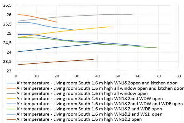
**Fig. 15** INDOOR AIR TEMPERATURE IN SOUTHERN LIVING ROOM WITH NATURAL VENTILATION AS A FUNCTION OF TIME (MINUTES)
