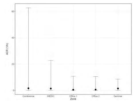
**Fig. 15** ESTIMATED DESIGN STAGE AIR CHANGE RATES FOR EACH BUILDING ZONE
