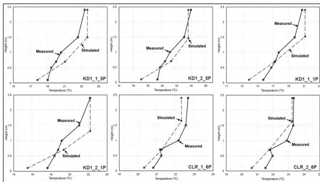
Fig.20 ENERGYPLUS THREE-NODE DV MODEL TEMPERATURE RESULTS COMPARISON.
