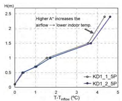
**Fig. 15** SHORT-TERM MEASUREMENTS :  $A^*$  IMPACT ON INDOOR AIR TEMPERATURE.
