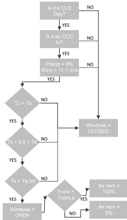
**Fig. 10** AUTOMATED WINDOW CONTROL FLOWCHART
