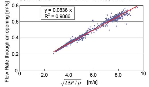
**Fig. 24** ΔP-Q CHARACTERISTICS OF THE NV OPENING
