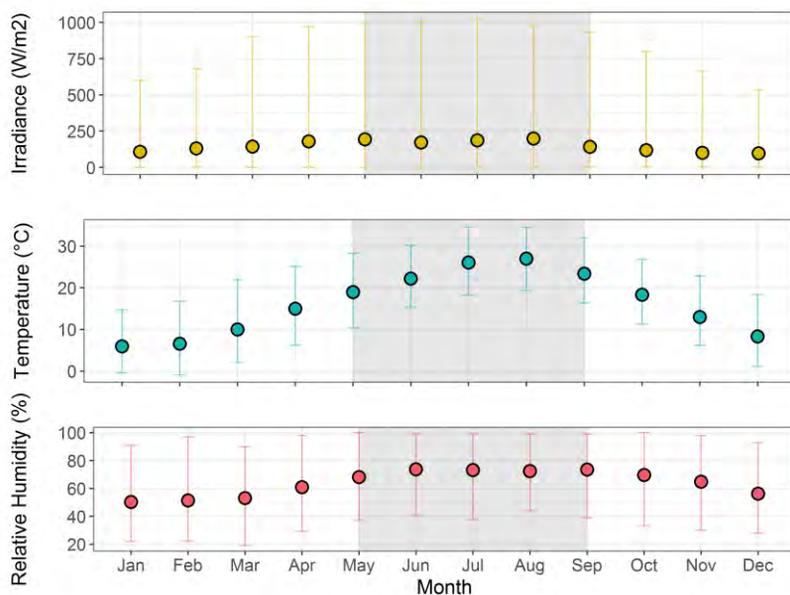
**Fig.2** LOCAL MEAN, MAXIMUM AND MINIMUM EXTERNAL CONDITIONS FOR KANAGAWA USING A TMY3 (AREA IN GREY IS COOLING SEASON)
