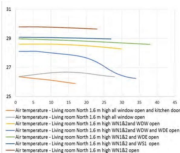
**Fig. 14** INDOOR AIR TEMPERATURE IN NORTHERN LIVING ROOM WITH CONCURRENT BALANCED AND NATURAL VENTILATION (X AXIS ARE TIME AND Y TEMPERATURES)
