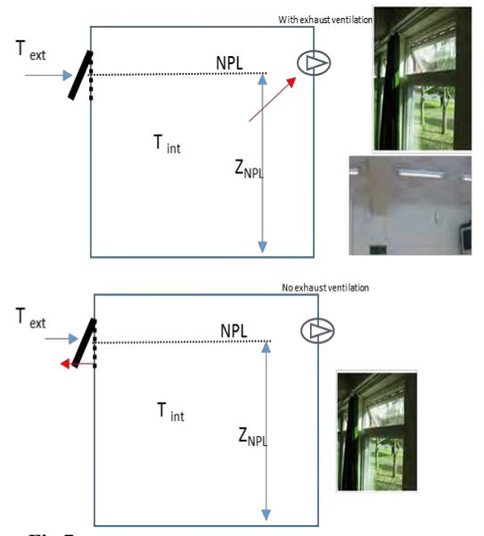
Fig.7 VENTILATIVE COOLING PRINCIPLE FOR HYBRID AND NATURAL VENTILATION
