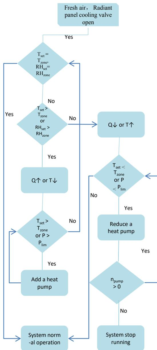
**Fig. 11** AUTOMATED CONTROL FLOWCHART
