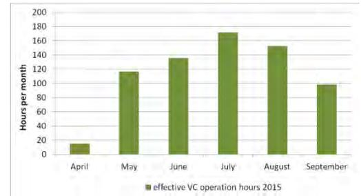
Fig. 19 OPERATION HOURS OF VENTILATIVE COOLING IN 2015
