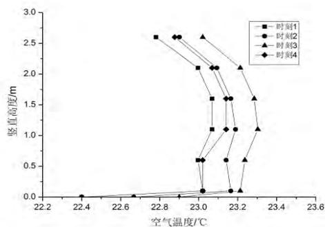
Fig. 16 INDOOR INDOOR AIR TEMPERATURE DISTRIBUTION IN THE VERTICAL DIRECTION
