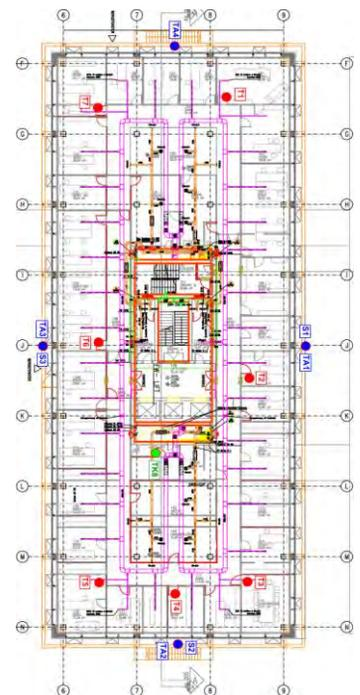
**Fig. 11** FLOOR PLAN WITH TEMPERATURE SENSORS, SOURCE: ATP ARCHITEKTEN INGENIEURE
