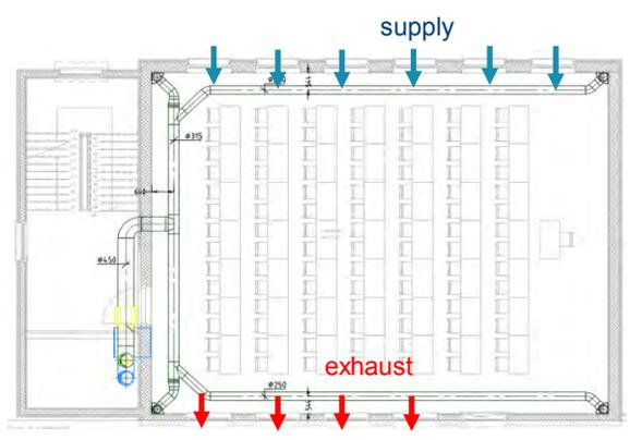
Fig. 9 PRINCIPLE OF NATURAL NIGHT VENTILATION
