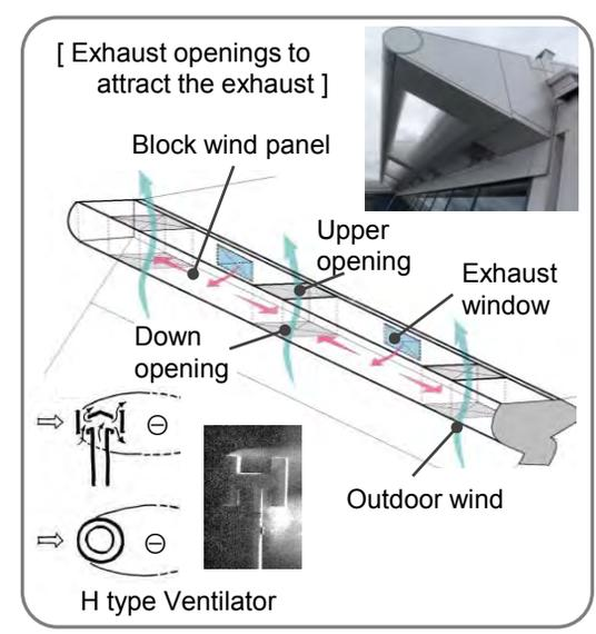
Fig. 17 SCHEMATIC DIAGRAM OF EXHAUST OPENING
