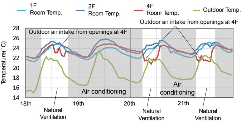
Fig. 25 4F ROOM TEMPERATURE FOR NATURAL VENTILATION IN MAY 2011
