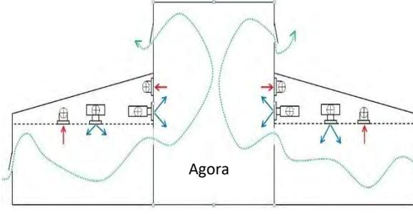
**Fig.10** NATURAL AND MECHANICAL VENTILATION PRINCIPLE
