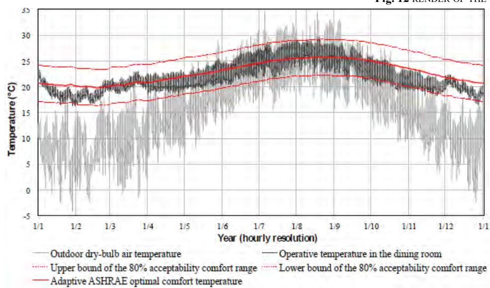
**Fig. 13** OPERATIVE TEMPERATURES INSIDE THE LIVING ROOM IN FREE-FLOATING MODE COMPARED WITH THE 80% ACCEPTABILITY RANGE OF THE ASHRAE ADAPTIVE MODEL.
