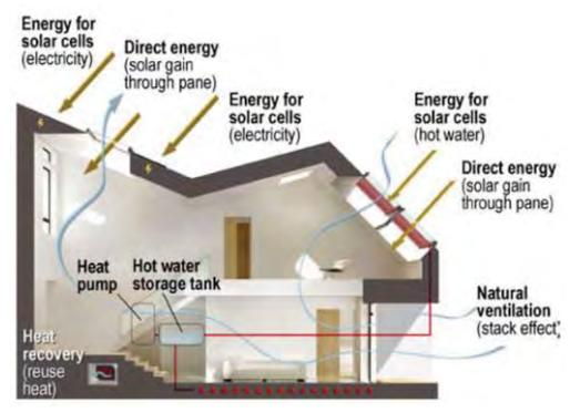
Fig. 8 VENTILATIVE COOLING PRINCIPLE
