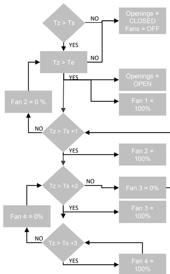
**Fig. 11** AUTOMATED OPENING CONTROL FLOWCHART
