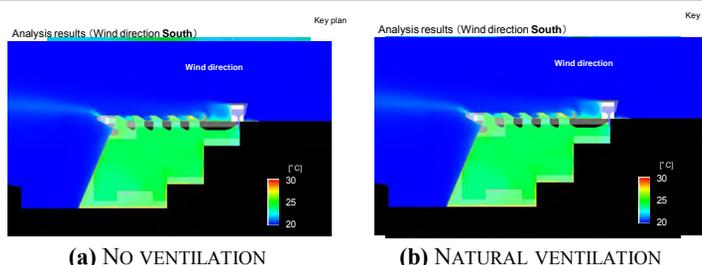
**Fig. 21** CONCEPT DESIGN STAGE SIMULATION: COMPARISON OF INDOOR THERMAL ENVIRONMENT FOR NATURAL VENTILATION
