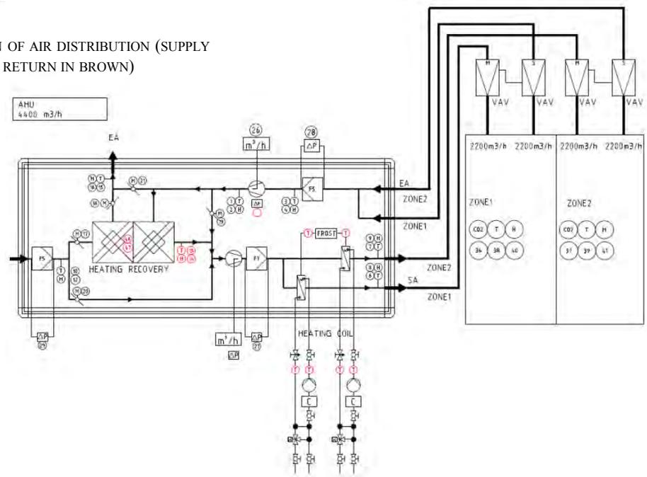
Fig.8 TECHNICAL DRAWING OF VENTILATION INCLUDING HEATING
