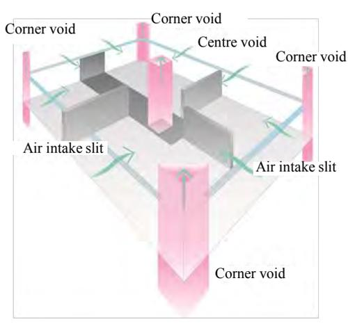
Fig. 16 SCHEMATIC OF NV AIR PATH THROUGH AN OFFICE ROOM
