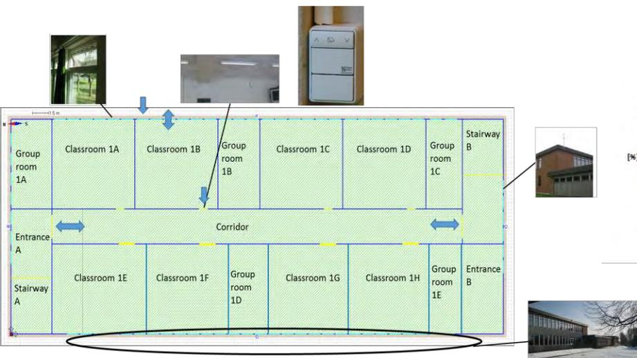
Fig. 9 HYBRID AND NATURAL VENTILATION AT BRUNLA. MOTOR CONTROLLED WINDOW AND EXHAUST TO A COMMON CORRIDOR
