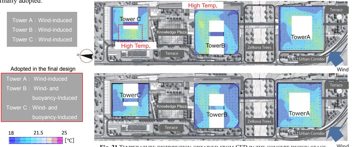
Fig. 21 TEMPERATURE DISTRIBUTION OBTAINED FROM CFD IN THE CONCEPT DESIGN STAGE
