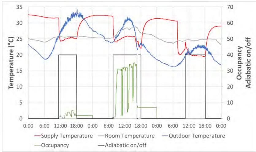
**Fig. 22** OPERATION INDIRECT EVAPORATIVE COOLING DURING AN EXTREMELY WARM PERIOD 21-23 JUNE 2017
