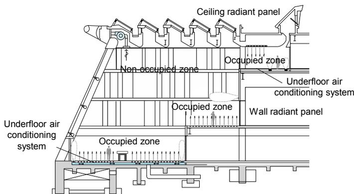
**Fig. 19** AIR CONDITIONING FOR OCCUPIED ZONE OF ATRIUM
