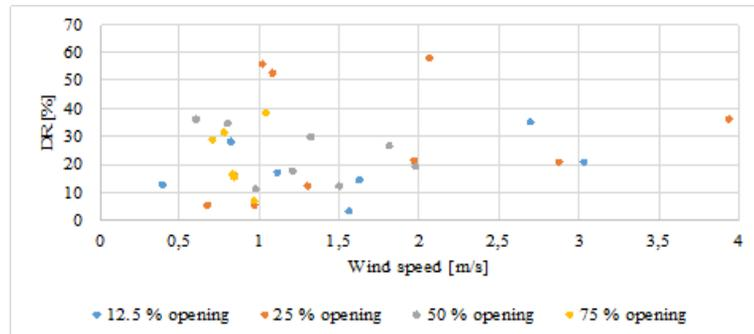
**Fig. 13 a)** TEMPERATURE DIFFERENCES BETWEEN THE JET AND THE ROOM **b)** DRAUGHT RATE FOR DIFFERENT WINDOW OPENINGS, BOTH (BLANDKJENN, 2016)
