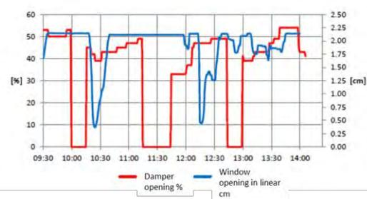
Fig. 8 DETAILS OF DAMPER AND WINDOW OPENING DURING OPERATION
