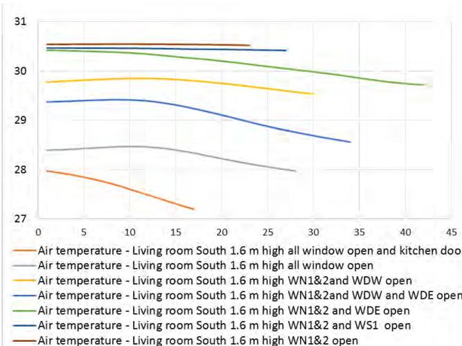
**Fig. 16** INDOOR AIR TEMPERATURE IN SOUTHERN LIVING ROOM WITH CONCURRENT BALANCED AND NATURAL VENTILATION AS A FUNCTION OF TIME (MINUTES)
