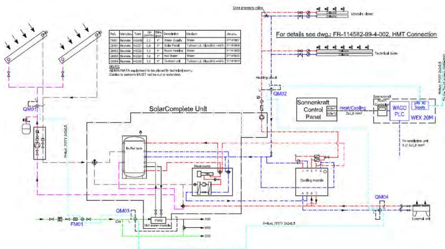
Fig.7 HYDRAULIC SCHEME OF HEATING AND HOT WATER SYSTEM
