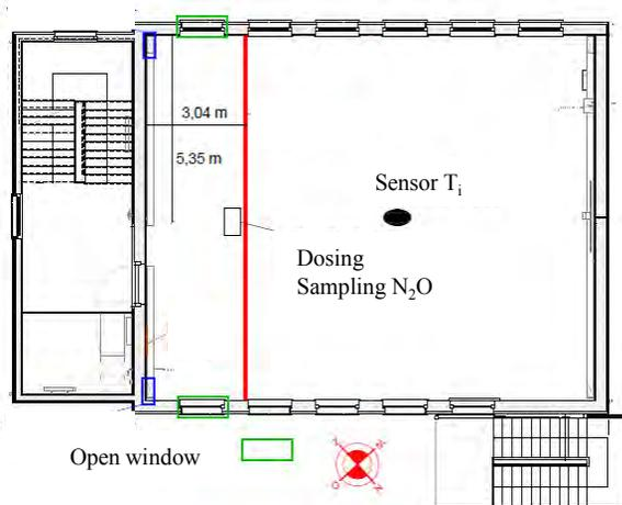
Fig. 17 Test set up tracer gas measurement
