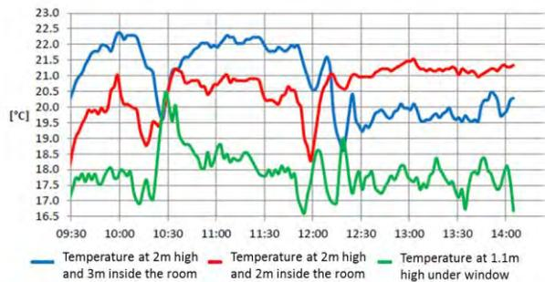
Fig. 16 INDOOR AIR TEMPERATURE FOR OUTDOORS TEMPERATURE OF 17 DEGREES AVERAGE
