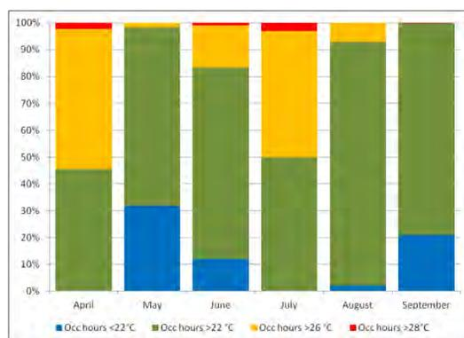
**Fig. 16** PERCENTAGE OF OCCUPANCY HOURS ABOVE THRESHOLD VALUES FOR INTERNAL TEMPERATURES IN ROOM 701 DURING 2015
