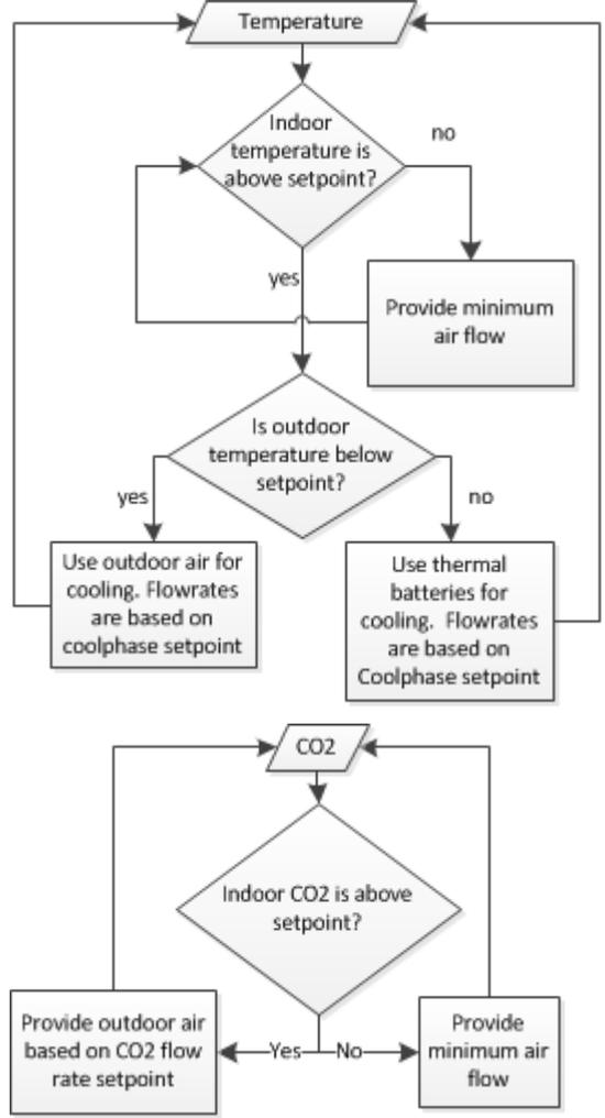
**Fig. 7** COOL-PHASE CONTROL FLOWCHART
