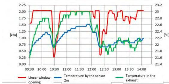
Fig. 14 TEMPERATURES VERSUS WINDOW OPENING
