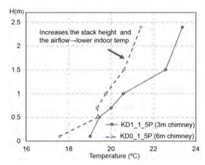
**Fig. 17** SHORT-TERM MEASUREMENTS : IMPACT OF CHIMNEY HEIGHT ON INDOOR AIR TEMPERATURE.
