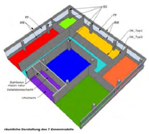
**Fig. 12** DESIGN STAGE SIMULATION OF RETROFITTED BUILDING USING DYNBIL, SOURCE: PASSIVHAUS INSTITUT.
