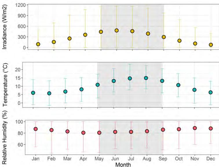
**Fig.2** MEAN, MAXIMUM AND MINIMUM EXTERNAL CONDITIONS IN CORK AIRPORT USING TMY3 FROM METEONORM 7 (COOLING SEASON SHOWN SHADED)
