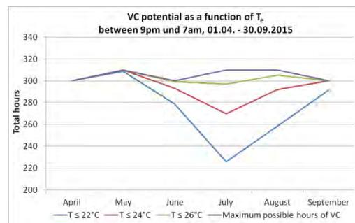
**Fig. 15** POTENTIAL FOR VENTILATIVE COOLING IN INNSBRUCK IN 2015 IN RELATION TO EXTERNAL TEMPERATURE
