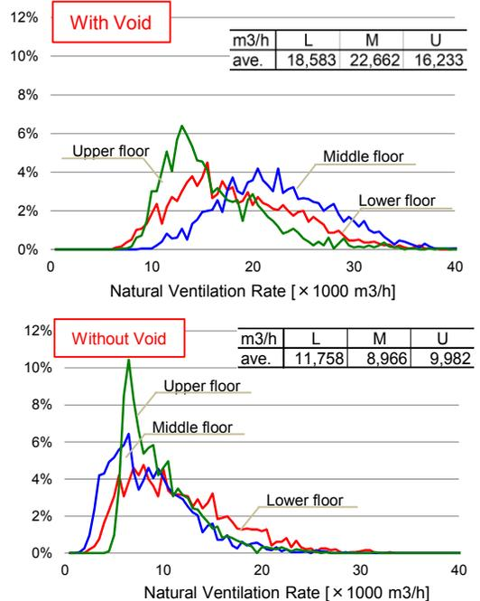
**Fig. 25** HISTOGRAM OF THE NATURAL VENTILATION RATE FOR THE CASES WITH/WITHOUT THE VOIDS
