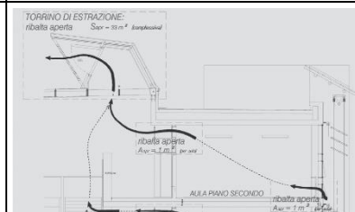
Image 03: Natural ventilation scheme © M.Grosso
