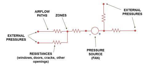
Figure 6-2. Schematic representation of relationship between zones and air paths. Source: IBPSA-USA
