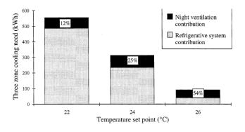
Figure 2.15. Daytime cooling needs of rooms A, B and C with and without night ventilation. [33].
