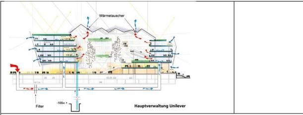
Figure 5.18. UNILEVER central administration building with exhaust atria, Hamburg, Germany
