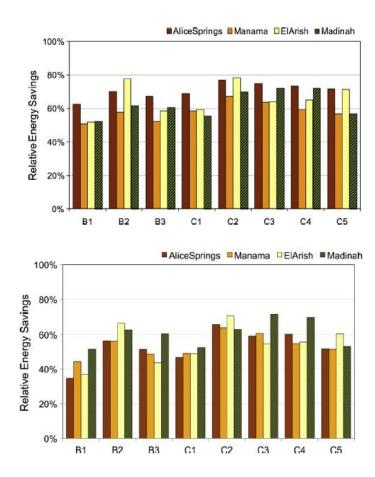
**Figure 2.17.** Savings in plant energy due to the application of hybrid cooling strategies for low (upper figure) and high (lower figure) internal heat gain relative to energy use of system B (VAV) [36].
