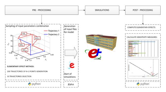
Figure 6.7. Sensitivity analysis procedure from sampling of input combinations by means of the elementary effect method to post-processing and sensitivity measures calculation. Source: Belleri A. [49]
