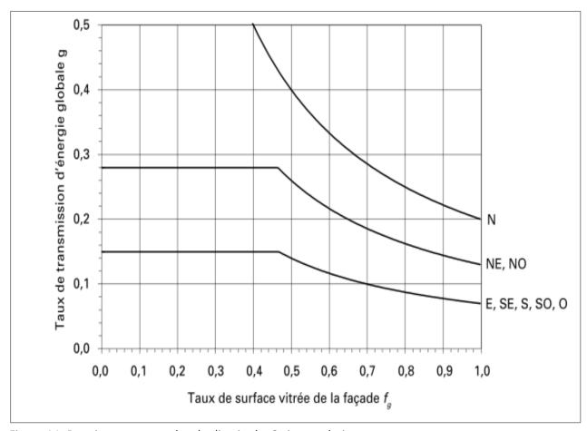
Figure A1: Requirements on solar shading in the Swiss regulations:
