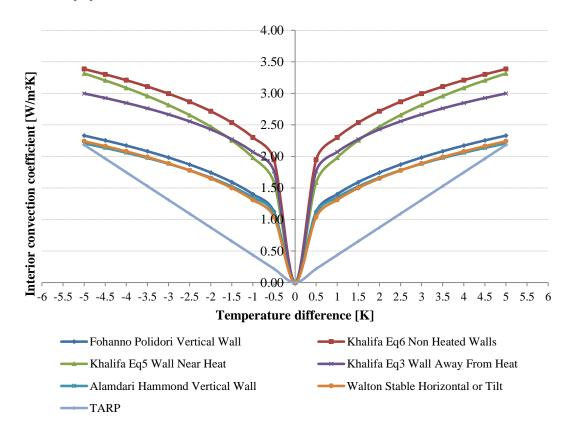
Figure 6-5. Vertical wall interior convection model comparison at different temperature differences between air and wall interior surface. Source: Belleri A. [49]
