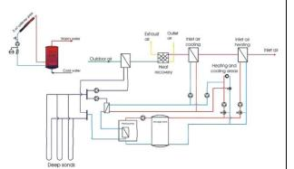
Schematic arrangement of the heating/cooling system
