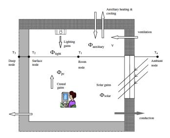
Figure 2.10. Illustration of a room thermal balance, [24].
