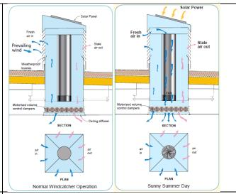
Figure 5.31. Modern fan-assisted, PV-integrated, bi-directional windcatcher by Monodraught, UK
