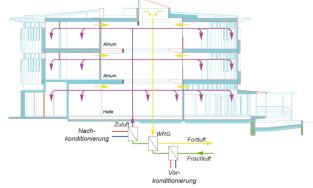
Schematic diagram of the balance mechanical air distribution system
