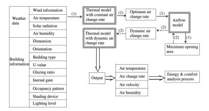
Figure 2.9. Structure of the two-coupled thermal and airflow model, [24].
