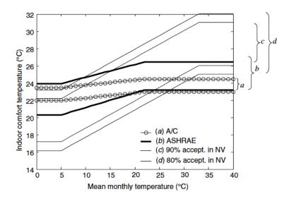
**Figure 2.2.** Comfort range for air conditioning and for natural ventilation: (a) air conditioning; (b) ASHRAE comfort range; (c) natural ventilation, 90% acceptability limits; (d) natural ventilation, 80% acceptability limits. [4].
