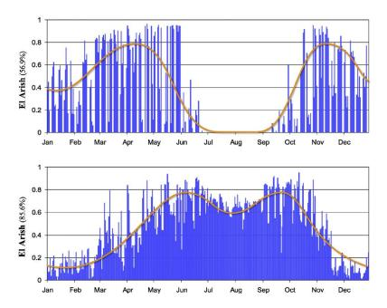
**Figure 2.18.** Window opening area of the optimal designs during the occupied hours and non-occupied hours. The annual proportion of night ventilation is noted in the vertical axis caption [36]
