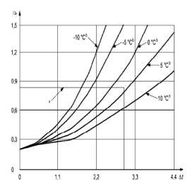
Figure 5.38. Chart of cooling effect from moving air, according to EN ISO 7730 [Source: ISO 7730:2005 Ergonomics of the thermal environment -- Analytical determination and interpretation of thermal comfort using calculation of the PMV and PPD indices and local thermal comfort criteria].
