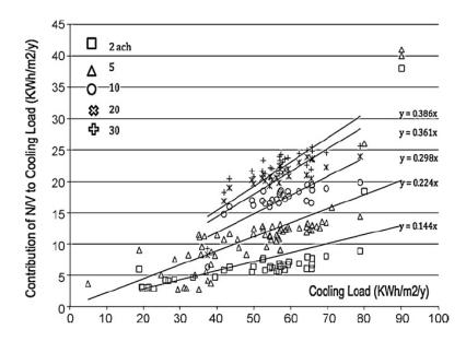
**Figure 2.19.** Calculated energy contribution of night-time ventilative cooling as a function of the initial cooling load for various levels of air flow rates, [37].
