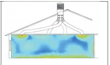
Figure 5.33. Modern bi-directional windcatcher with option for ducted air dispersal by Passivent, UK
