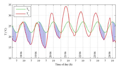
**Figure 2.4.** Building temperature, T<sub>b</sub> and external air temperature, T<sub>e</sub> during one week in summer 2003 for Zurich SMA (ANETZ data). Shaded areas illustrate graphically the climatic cooling potential, CCP. [13]
