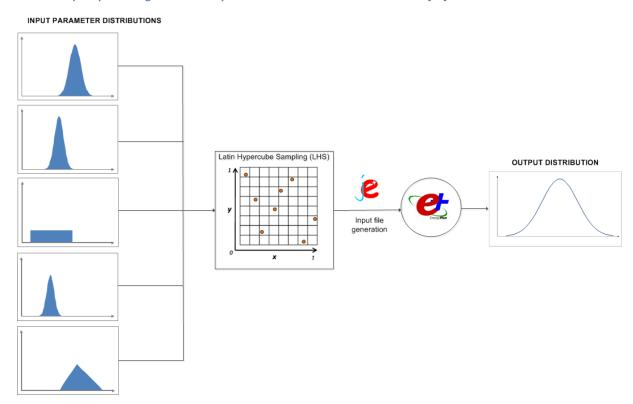
Figure 6.8. Uncertainty analysis procedure from input parameters probability distribution assignment, to sampling by mean of the Latin Hypercube method to post-processing and output probability distribution. Source: Belleri A. [49]
