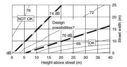
**Figure 2.12.** Contours of noise level at different heights above the street and street widths. Configurations in which natural ventilation is possible are indicated (OK), as are those in which it is ruled out (NOT OK). Between these two extremes is a region in which there are possibilities for design solutions. [30].
