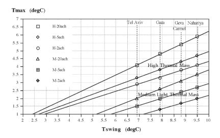
Figure 2.20. The reduction in Tmax in the hot-humid climate of Israel, as a function of Tswing, [38].
