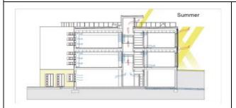
Cross and vertical ventilation systems acting together with the buried pipes system
