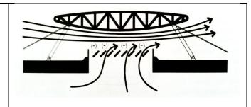
Figure 5.22. Principle of Venturi ventilator with adjustable louvres system. Source: [21]
