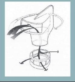
Figure 5.35. Two examples of windscoops, first one: Exhaust windscoop system Kaufman (also addressed as deflector), USA, Source: www.scoopsandrakes.com, second one: scematic sketch of a modern intake windscoop. Source:
