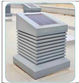
Figure 5.30. Modern windcatcher Sola-Boost by Monodraught, UK. It is devided into four sections, working bidirectional at all wind directions. Integrated there's a 10W monocrystalline photovoltaic solar module, linked to an assisting fan (2W at nominal power), adding up to 35I/s in addition to 110I/s ventilation calculated at between 2 and 3 m/s external wind speed. Source: http://www.monodraught.com (20.04.2014)
