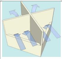
Figure 5.29. Traditional windcatcher at Qatar and sketch of functional principle
