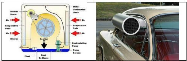
Figure 5.41. Principle of a swamp cooler and example of a historic car swamp cooler . Source: www.teachengineering.org (04.01.2015) and historic example of a car swamp cooler. Source: www.etsy.com/de/listing/115395443/swamp-cooler-vintage-fenster-ac (05.01.2015)
