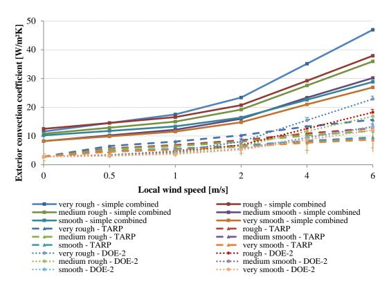
Figure 6-4. Vertical wall exterior convection model comparison depending on wind speed and surface roughness at a temperature difference of 10K between outdoor air and external wall surface when the façade is directed windward. Source: Belleri A. [49]
