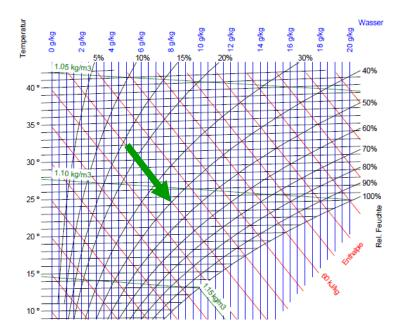
Figure 5.40. Process of evaporiative cooling within the psychrometric chart
