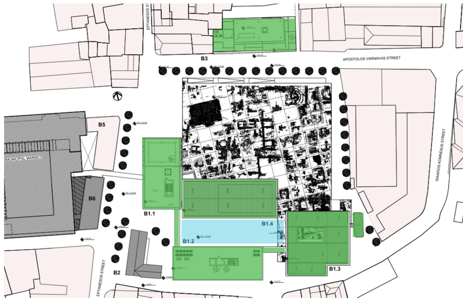
Figure 1: Instead of a single building occupying the whole land, a family of small buildings around the archaeological findings create interesting bioclimatic potential
