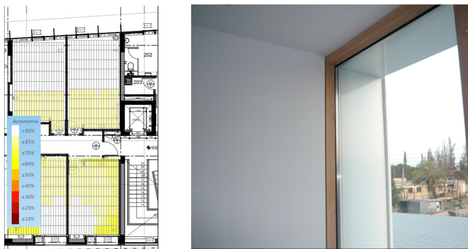
Figure 8: Natural light autonomy, simulated with DIAL+ software between 75 and 85% during working hours
