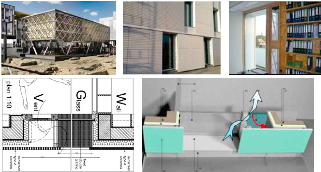
Figure 2: The Nicosia Townhall where special façade vents were developed to realise ventilative cooling in the building [2]
