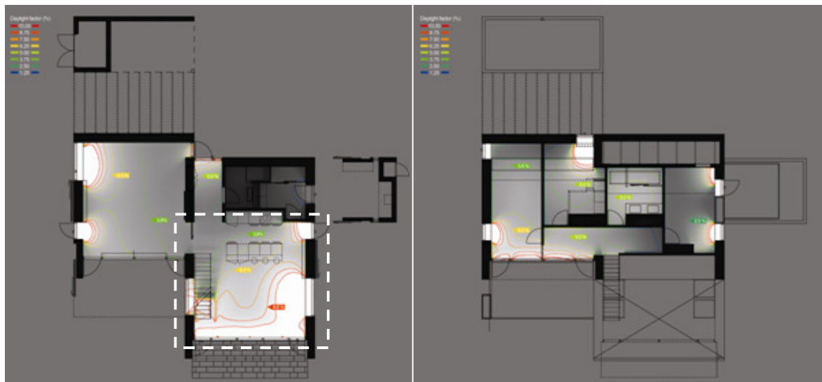
Figure 2: Calculated daylight factors in “Home for Life”. Ground floor on the left, and upper floor on the right. The dotted rectangle indicates the kitchen and dining room which will be investigated in details.
